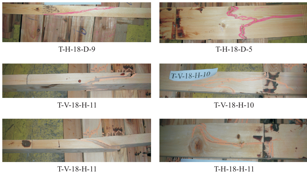
Fig. 5. Failure due to knots and the grain slope of finger-jointed lumber in tensile testing.
