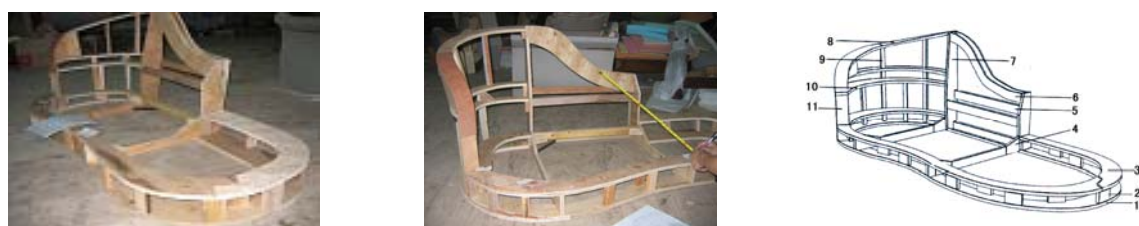
1-seat frame down layer plate 2-seat frame column plate 3-seat frame up layer plate 4-seat frame cross-file plate 5-backrest cross-file plate 6-backrest top plate 7-backrest column plate 8-handrail top plate 9-handrail column plate 10-handrail cross-file plate 11-handrail front plate
