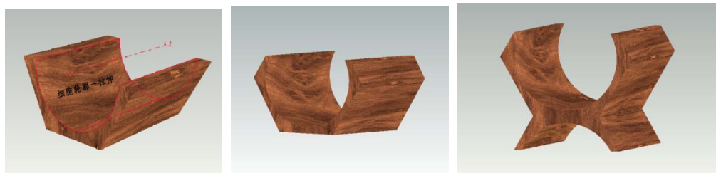
Fig. 3 The cross-section shape of wood cracking fiber.
