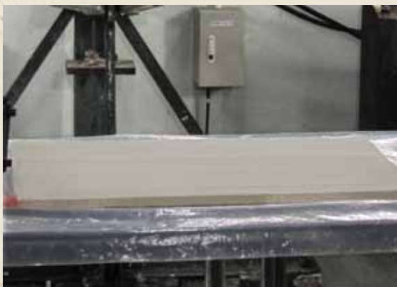
壓榨完成之紙堆 Paper stack after pressing.
