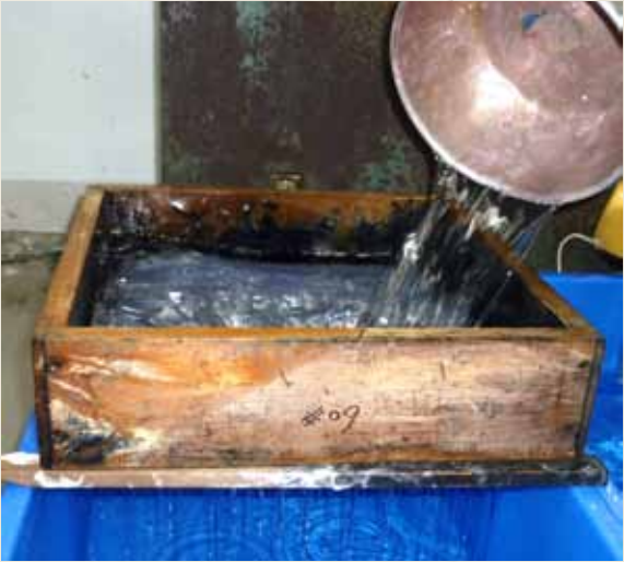
分散劑過濾 Filtering dispersant to remove lumps.
