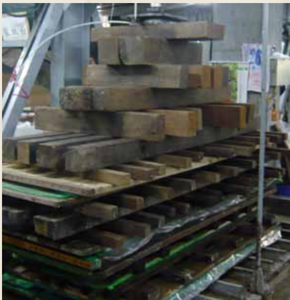
壓榨去水 Pressing dewatering.
