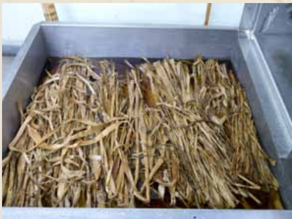
原料蒸煮前浸泡處理 Soaking of the raw materials before digestion.
