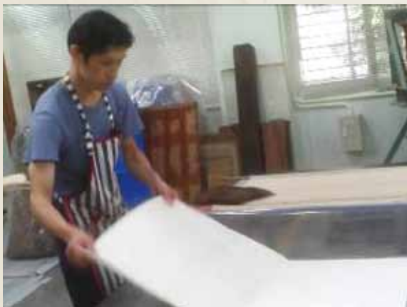
紙張烘乾 (3) Drying by a large heated platen(3).
