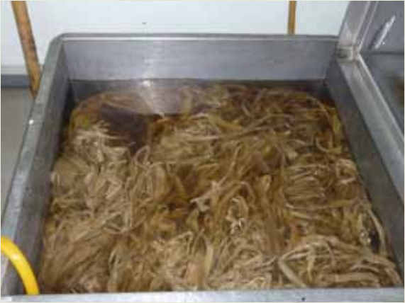
原料清洗 Washing of the cooked raw materials.
