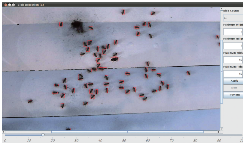
Fig. 1. A graphical user interface showing the image with a colored square around the recognized blob and the automatic process of counting the number of bees.
