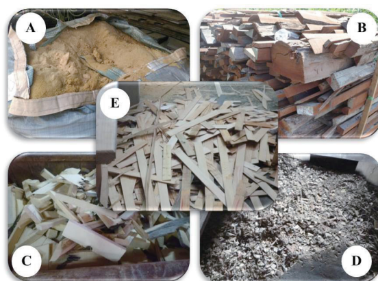
Fig. 1. Types of woody wastes. (A) Sawdust; (B) bark waste; (C) sawn timber; (D) woodchips; (E) wood leftovers.
