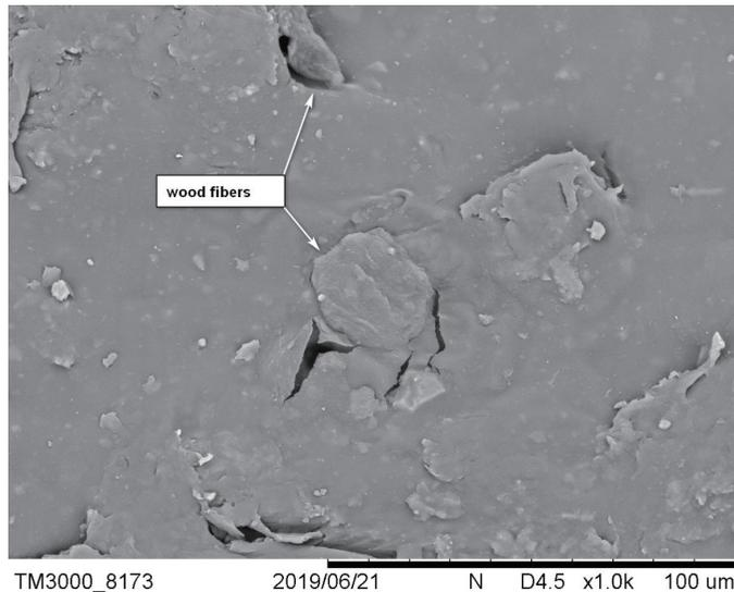
**Fig. 3.** SEM image of a specimen showing clear gaps between the wood flour (WF) and polylactic acid (PLA) interfaces.
