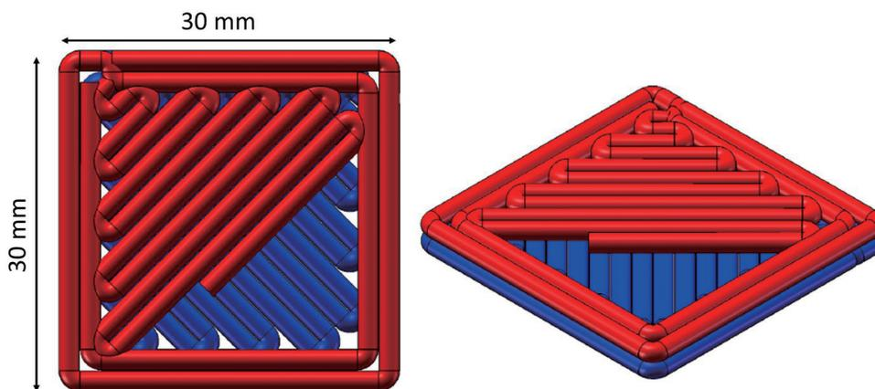
Fig. 1. Schematic representation of a printed cuboid specimen.
