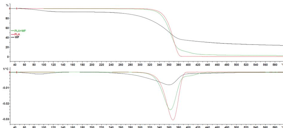
**Fig. 2.** Thermogravimetric analysis (TGA)-DTG curves of wood flour (WF), polylactic acid (PLA), and the WF/PLA composite (PLA+WF).
