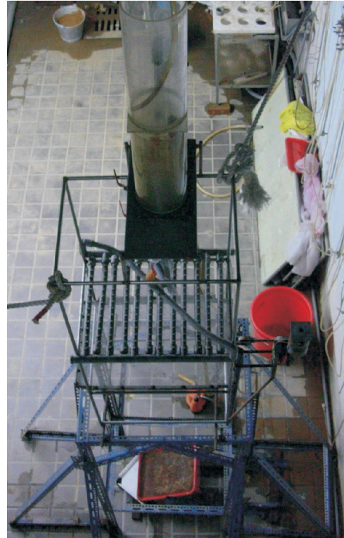
Fig. 2. Artificial rainfall simulator.
