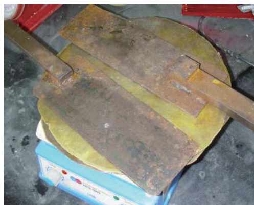
Fig. 1. A set of self-made copper heating plates.
