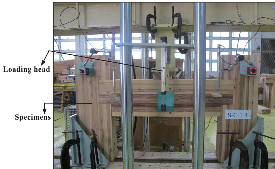
Fig. 2. Japanese cedar glulam beam-column set-up and test apparatus to apply a concentrated load for the shear resistance of the connection.
