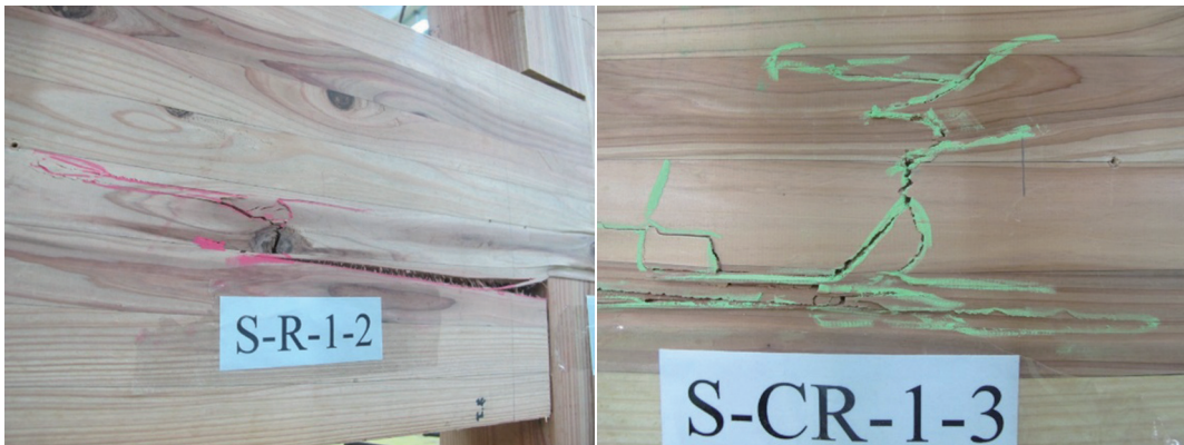
Fig. 8. Split failure at the notch corner and shearing failure at the center of a Japanese cedar glulam beam member.
