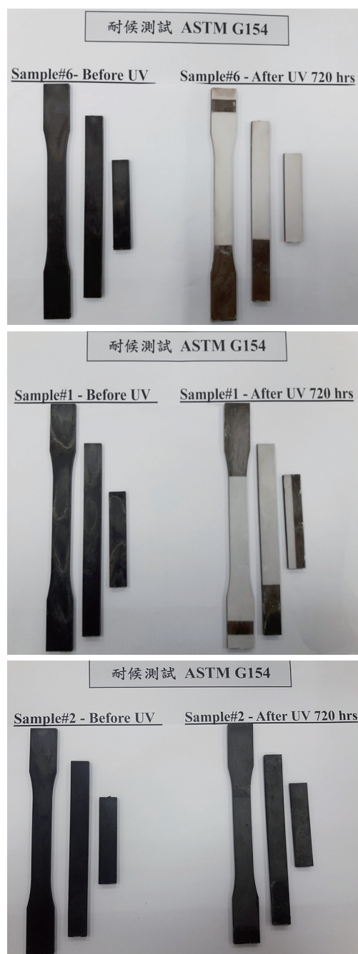
Fig. 2. Photographs of wood-plastic composite test specimens (WPC-TSs) prior to and after the weathering test. Top image (WPCs-1~16); central image (WPCs-17~20); bottom image (WPCs-21, -22).
