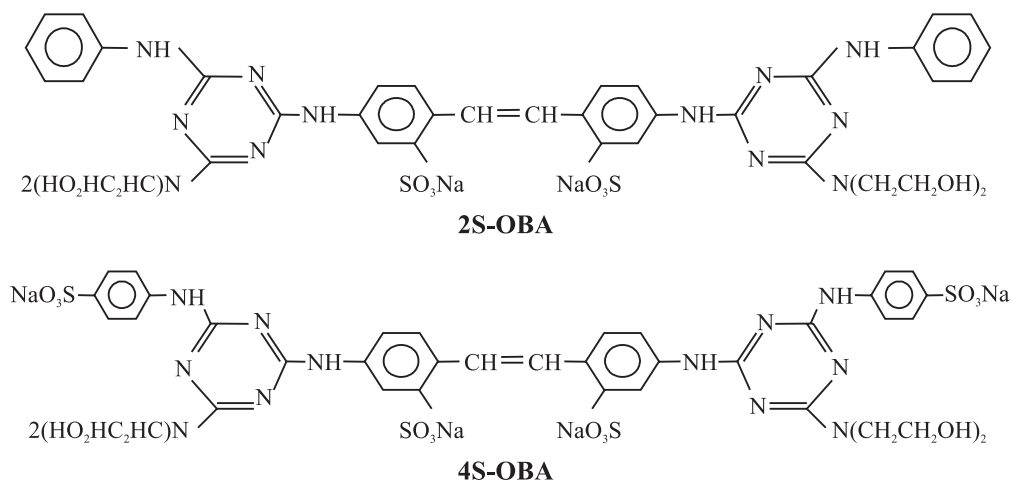
Fig. 1. Chemical structures of 2S- and 4S-optical brightening agent (OBAs).
